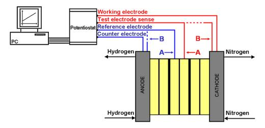
Fig. 6. Potentiostatic assembly dedicated to the fuel crossover measurements for one individual cell in the FC stack (A) and for the whole FC generator (B).
