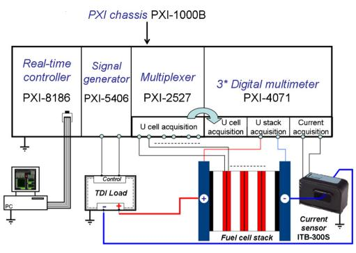
Fig. 1. Scheme of the experimental EIS measurement system developed in-lab.
