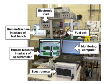
Fig. 2. Impedance spectroscopy measurement on a PEMFC stack.
